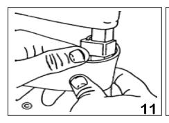
(Front view) Using heavy thumb pressure of one hand hold strap in position and begin wrapping strap around frame with your other hand. Slide clip onto frame. me. As shown in (Pic.11)
