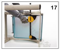
A spreader tool is needed and you can find it on our website under tools. Turn the chair upside down and put the spreader tool in the rails behind the chair; doing so will help to stretch the fabric. Note: The fabric was made to stretch up to 1 3/8". See (Pic.17)
