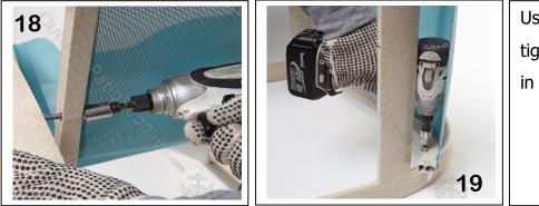
Use an impact drill to tighten all bolts as shown in (Pic.18 and 19)
