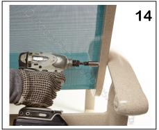
On the side that is still attached to the frame, loosen all bolts <sup>3</sup>/<sub>4</sub>" of the way using an impact drill as shown in (Pic.14)
