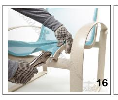
Pull the sling until it is even with both ends of the rails, and if necessary, use pliers to eliminate wrinkles on the fabric.
